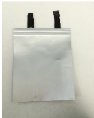
Thermoconformable LIB cell with CNT current collector and Polymer electrolyte
